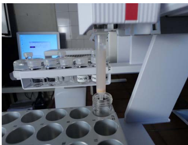
Fig. 1. SPE-cartridge after aspiration of sample from the opening on the bottom.
