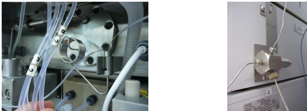
Fig. 2. Left : Parts of a standard Agilent system: mixer is the packed steel column (built in horizontally on the left), which was exchanged in our system by the round filter based mixer (see Fig. 1). The column-type mixer has an even larger dead volume (approx. 600 \mu L). Right : Shimadzu mixer and tubing (from mixer to column): dead volume approx. 100 \mu L
